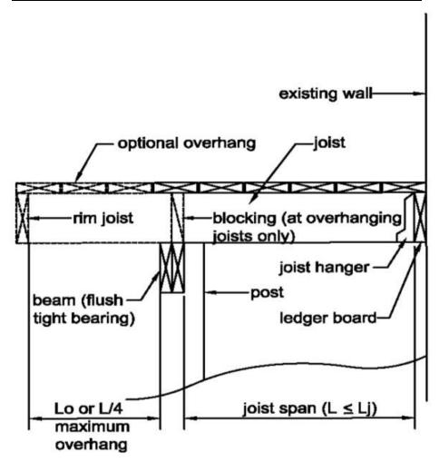
The joist span is the distance between the two points supporting the joist (i.e. ledger to beam, beam to beam) and does not include any overhang. Allowable cantilever is joist span = (L)/4.
