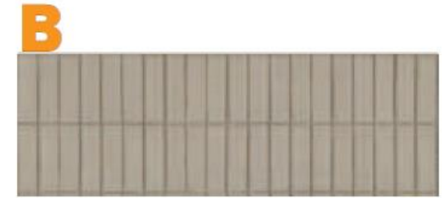
MATERIAL: MODULAR BRICK PATTERN: SOLDIER COURSE (VARIES) FINISH: PAINTED SW 7017 DORIAN GRAY
