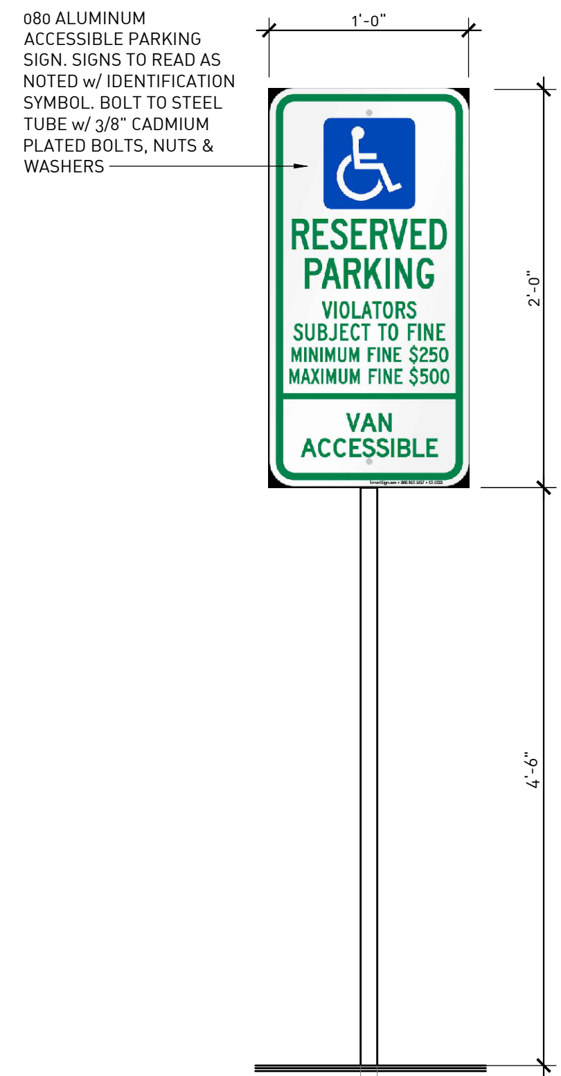
ACCESSIBLE PARKING SIGN DETAIL 5 spt.1 NO SCALE
