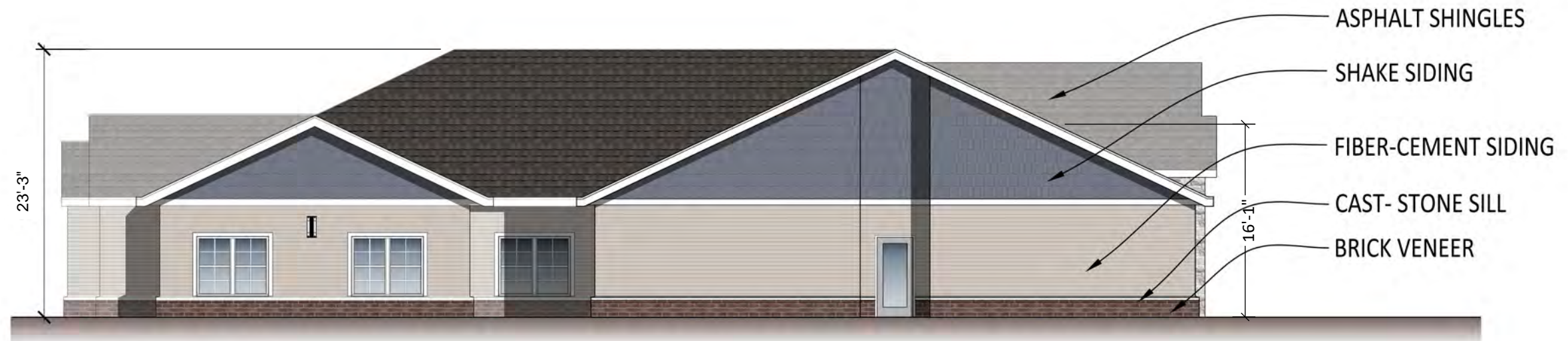
WEST ELEVATION 3/32" = 1'-0" SIDE
