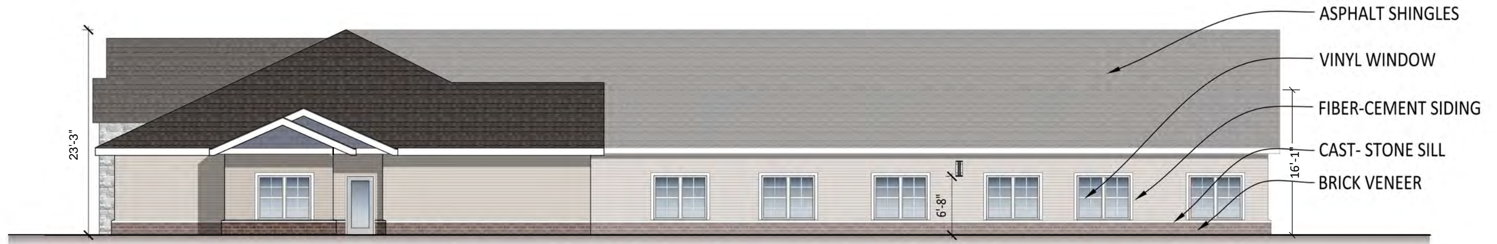
NORTH ELEVATION 3/32" = 1'-0" FRONT
