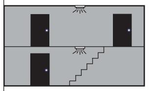
disconnect the power source. Simply fan the smoke away from the detector until the alarm stops. If this happens frequently, it may be necessary to relocate the detector or to install a different type of detector.
