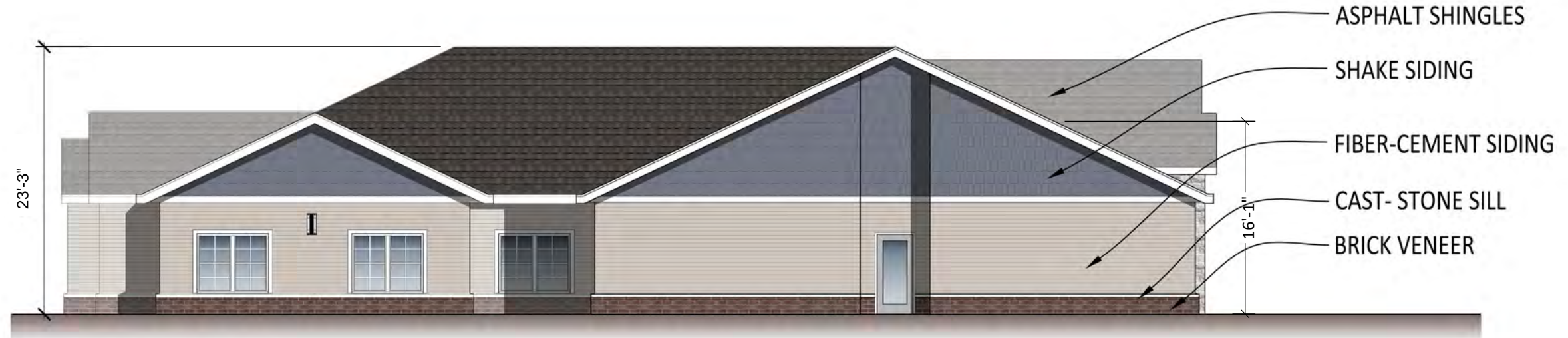
WEST ELEVATION 3/32" = 1'-0" SIDE
