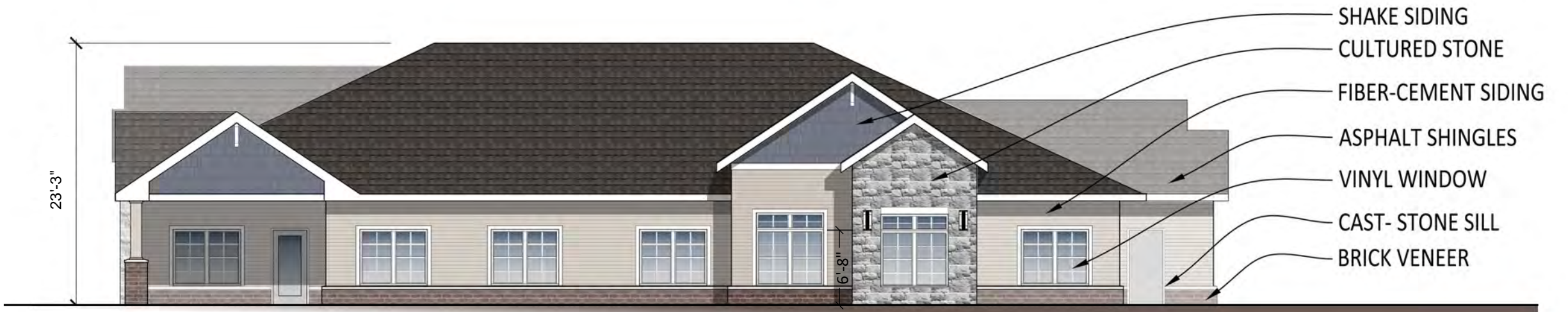
EAST ELEVATION 3/32" = 1'-0" SIDE
