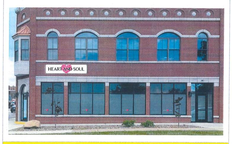
DESCRIPTION: 144" x 34" Routed 6mm MaxMetal Sign with 123" x 11.25" x .5" Raised PVC Letters and Digitally Printed and Laminated Vinyl Background Graphics (1)
