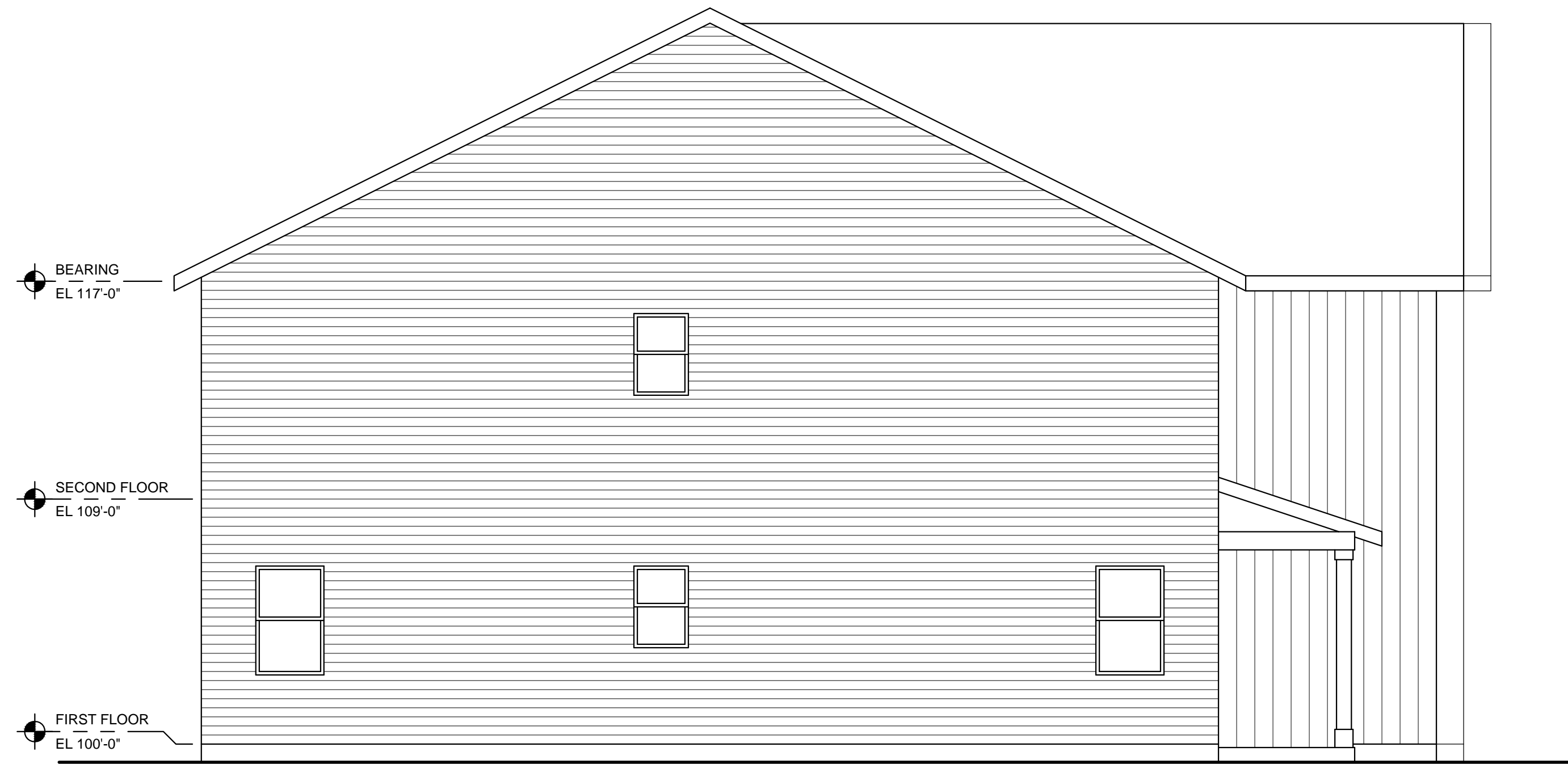
2 EAST ELEVATION A-200 1/4" = 1'-0"
