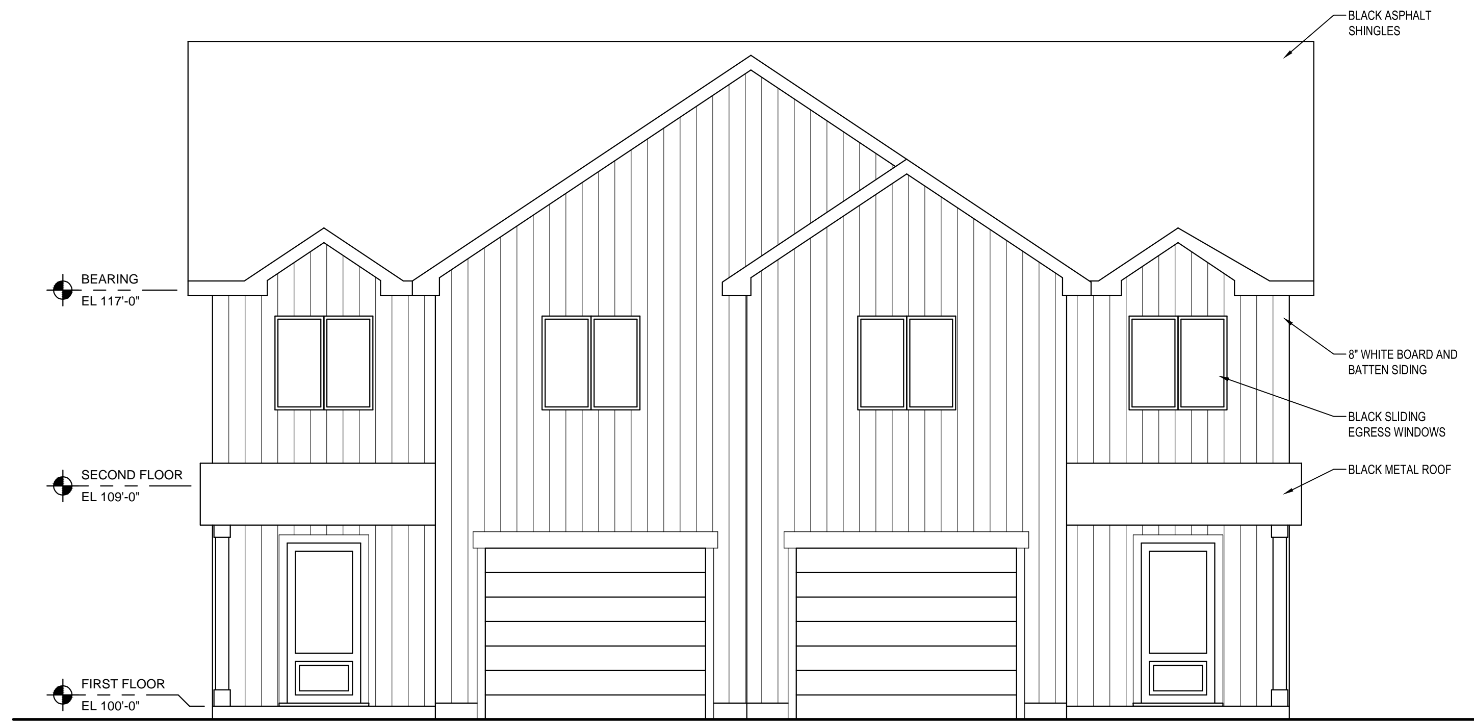
1 NORTH ELEVATION A-200 1/4" = 1'-0"
