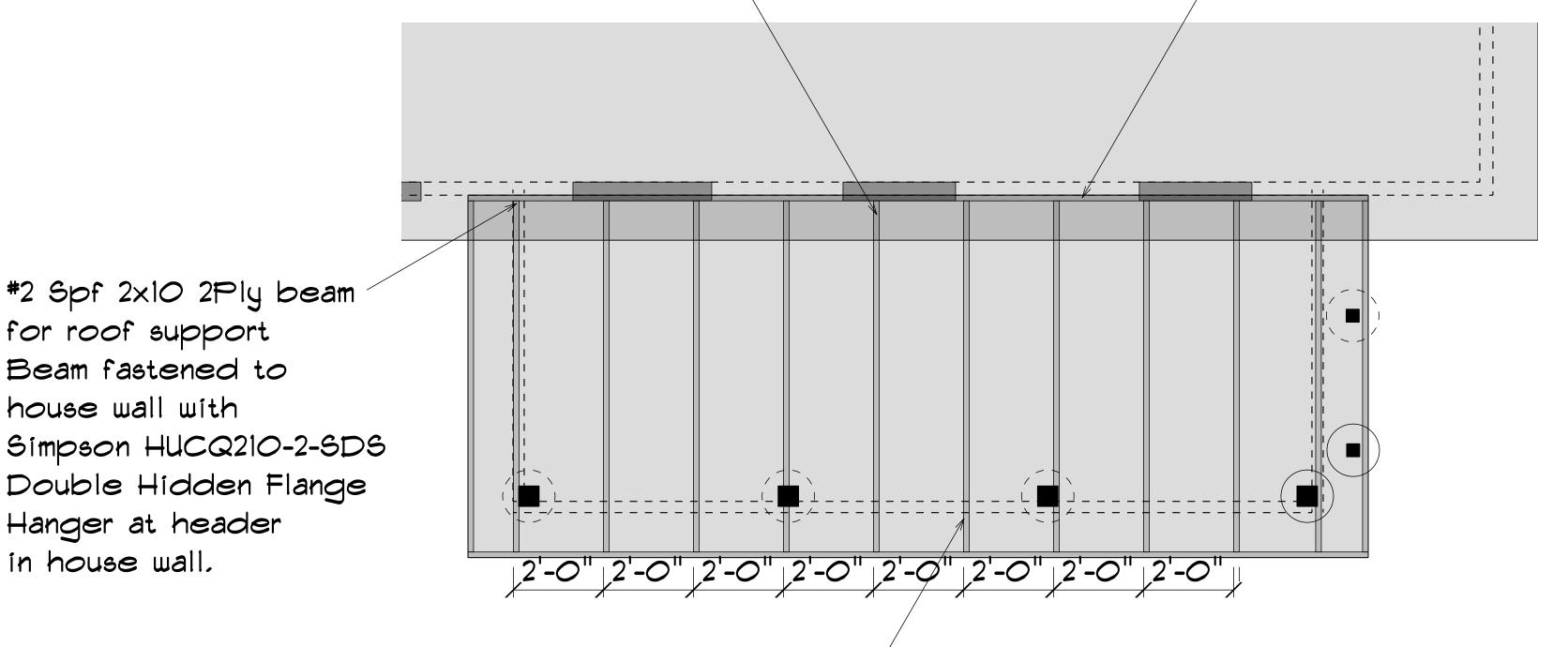
Rafters fastened to beam with Simpson H-2.5A Rafter Tie Down
